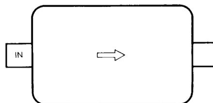
Flow Direction – Liquid Line Drier
