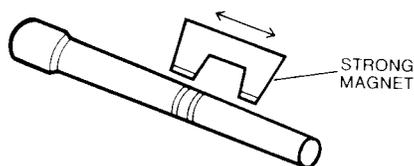
Testing Check Valve With A Magnet
