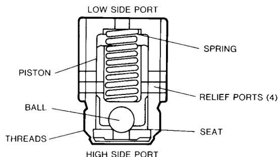
Compressor Internal Pressure Relief Valve
