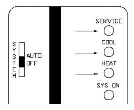
SIMULTANEOUS BLINKING - Supply Air High Limit Duct Static Trip. Manual Reset. (27.5-50 ton VAV only)
