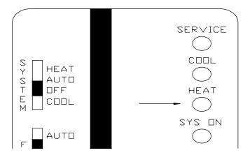
**ON**-Indicates unit is in the heat mode, and actively heating. **BLINKING**-Indicates a Heating Failure has occurred. **OFF**- Indicates that the unit is "not" actively heating.
