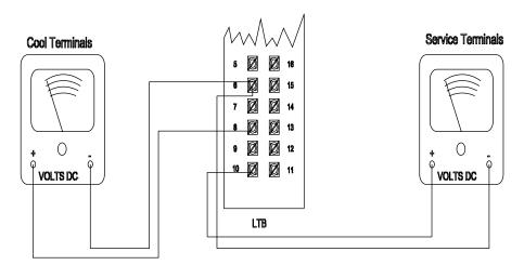
**LTB-6 & LTB-10 Failure** = Alternates between 32 VDC & 0.75 VDC. **LTB-6 & LTB-8 Failure** = Alternates between 32 VDC & 0.75 VDC.
