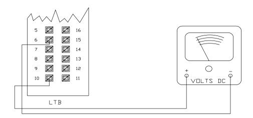
Clogged Filter (CFS)/Fan Failure (FFS) (3-25 only) = Approximately 32 VDC. Indication only.
