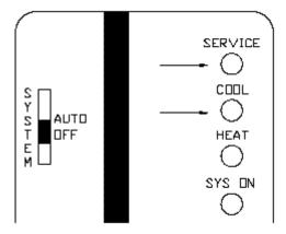
SIMULTANEOUS BLINKING - Static Pressure Transducer Failure (27.5-50 ton VAV only)
