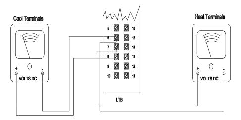
**LTB-6 & LTB-8 Failure** = Alternates between 32 VDC & 0.75 VDC. **LTB-6 & LTB-7 Failure** = Alternates between 32 VDC & 0.75 VDC.
