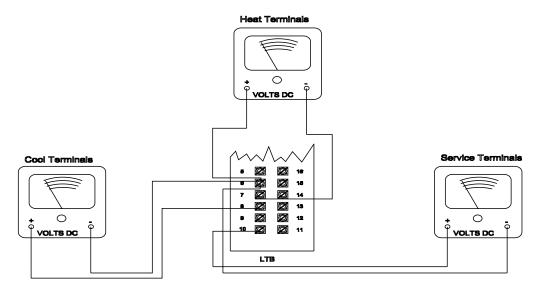
LTB-6 & LTB-10 Failure = Alternates between 32 VDC & 0.75 VDC.
