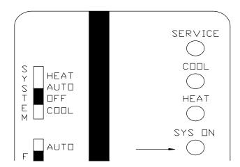
**ON**-Indicates that the UCP is powered up, also indicates that the software/computer program is intact and functional, and is lit continuously during normal operation.
