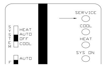
**ON**-Indicates Clogged Filter (CFS) or Fan Failure (FFS) (3-25 ton only), indication only. **BLINKING**-Indicates Active Fan Failure (AFF) (3-25) or Fan Failure (FFS) (27.5-50 ton only), unit shuts down. **OFF**-Neither of the above have occurred, or not being used.
