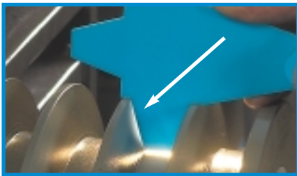
Worn Groove Sidewalls
