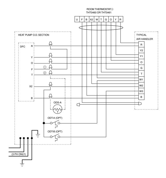
① Installations not using DFC service light feature, **MUST** have "F" wire (RD/WH) jumpered to "R" wire (RD) in O.D. unit. Do **NOT** use for installations with variable speed O.D. compressors.
