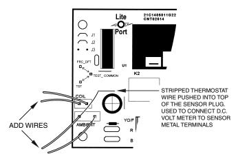
Connect a D.C. Volt meter to the stripped wires and read the voltage. Determine the sensor's temperature and compare the voltage taken to the Defrost Board Sensor Table. If they are within plus or minus 15 percent, the sensor is OK. If the readings are out of range or no voltage reading, proceed as follows:
