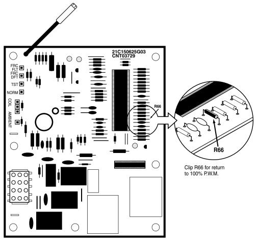
A new defrost control has been introduced for the two compressor heat pump series of units. The control, part number CNT03729 (Dwg. #C150625G03), will be compatible with the existing controls.
