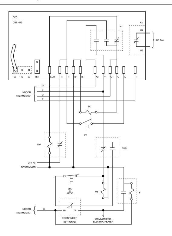
EDR relay energized in the cooling cycle only, so EDC thermostat will be in the circuit. EDC or LPCO must be bypassed during defrost cycle.
