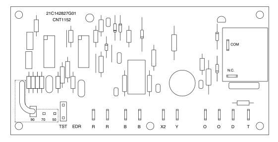
• CNT1152 is NOT furnished with EDR control terminal and may be replaced by CNT1642
