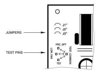
Wire Jumpers J1, J2 and J3, will be replaced in the future with Ø ohm resistors.
