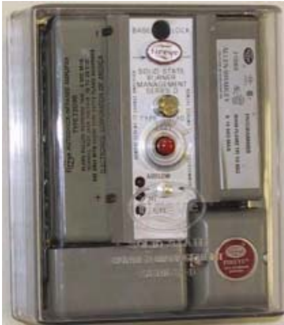
Fig. 46 D Series control chassis with program module and amplifier installed.
