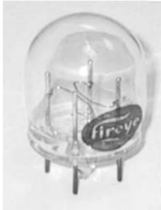
Fig. 10 UV radiation detection tube. Fireye part no: 4-320
