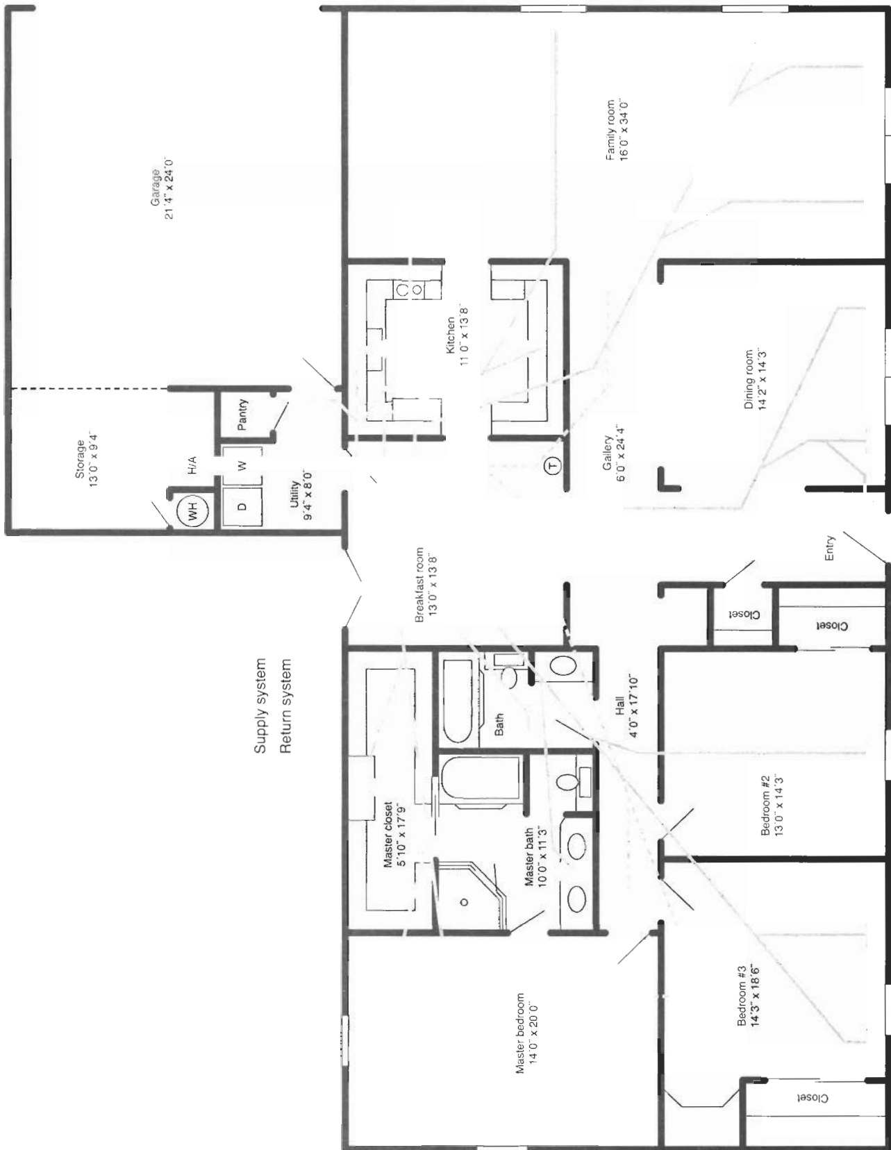
Figure 6. Large single-floor residence with floor distribution system and indoor unit in garage
